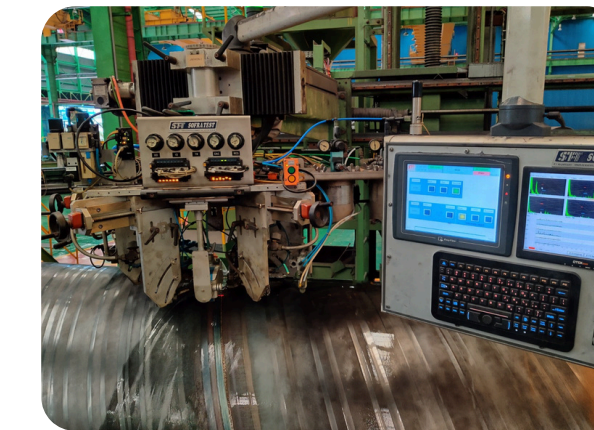
SSAW ON-LINE WELD INSPECTION
