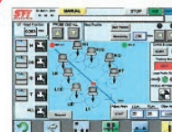
WELD INTERNAL 70° EXTERNAL 70° HAZ 25 mm
